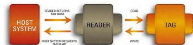
Figure 2: Basic component of RFID system
