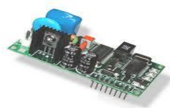
Figure (3): PLC Modem
